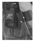
Insert the control box into the hipmount bag. Then insert the connector (female) in its panel connector (male) and screw it.
