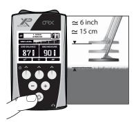
On the controller, press the "Ground Balance" button 💿 once briefly **while** pumping the coil to the ground. The ORX will grab and calibrate the current ground value and stabilise your ORX. The number on the lower left of the screen (GND BALANCE) displays the users set ground value.
