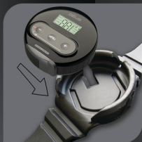
Lodge the headset control inside the wristband*
